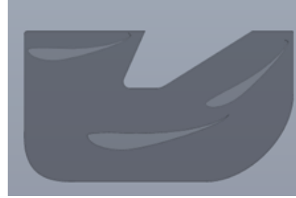
Fig. 33 Cross sectional view of rear wing, second design
