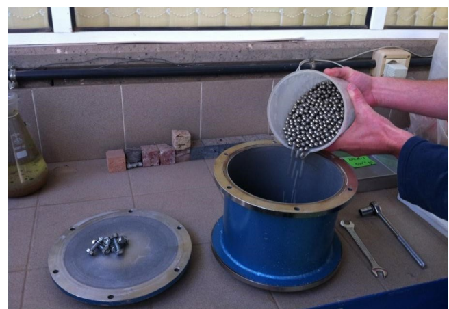
Figure 2. Introduction of the abrasive load (5,000 g of steel balls) in the Micro-Deval cylinder
