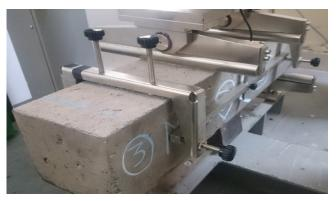
Figure. 1. Flexural testing on beam.
