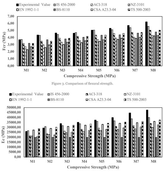
Figure 4. Comparison of Modulus of Elasticity.
