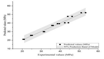
Figure 6. Comparison of cylinder compressive strength.
