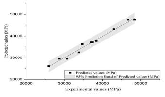
Figure 8. Comparison of modulus of elasticity.
