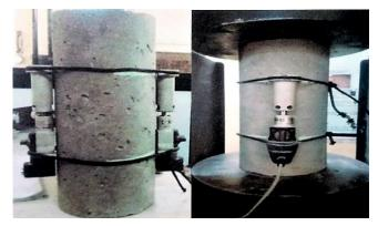
Figure 2. Modulus of elasticity test on cylinder.
