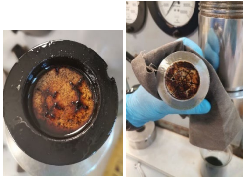
Figure 11: Precipitate at Limestone Core-Head
