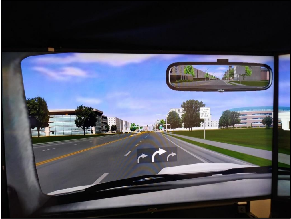
Figure 5.8: An illustration diagram is shown 700 feet upstream the stop line at the main intersection
