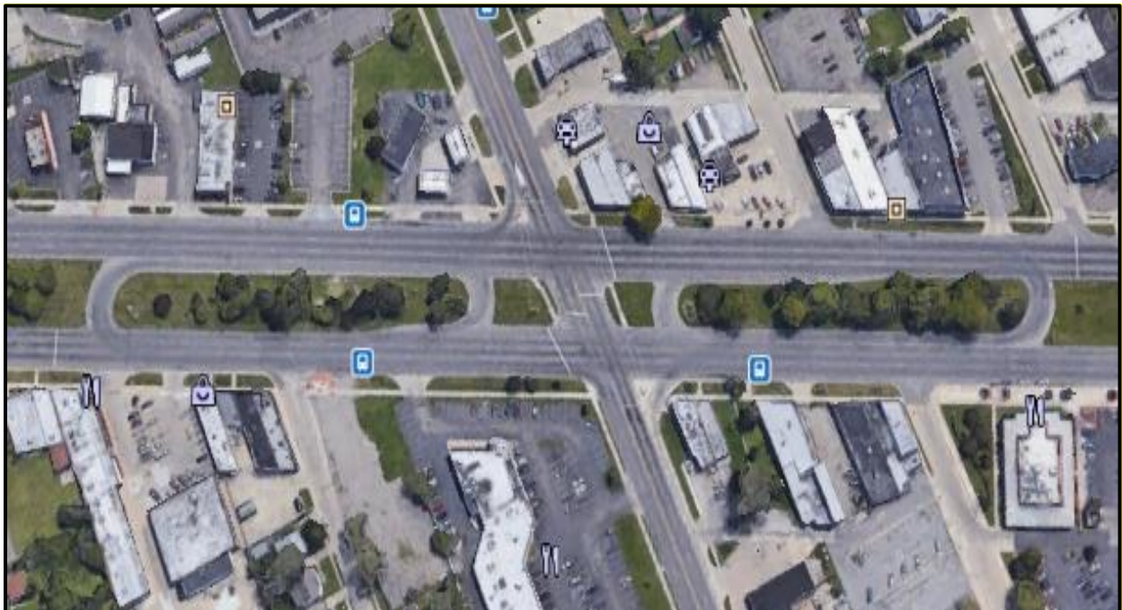
Figure 3.2: MUT type B intersection at E 10 Mile Rd and Gratiot Ave., Eastpointe, MI ( Google Earth )
