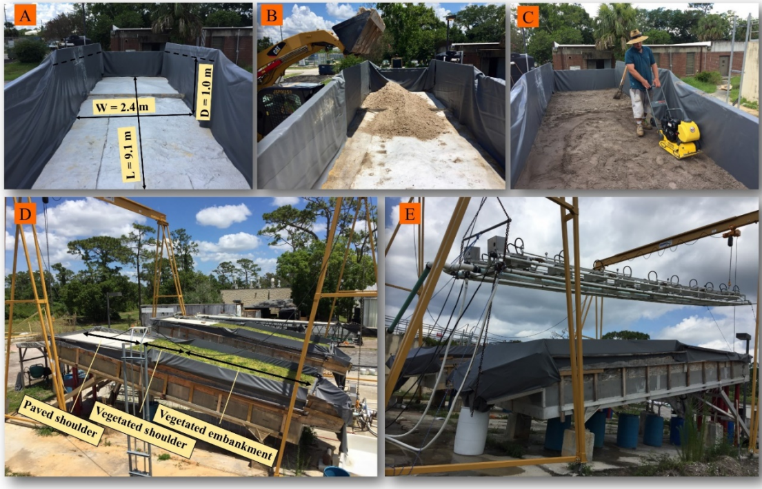
Figure 3. Model construction and dimensions (A), filling with the media (B), compaction (C), final design with established vegetation (D), and hoisted calibrated rainfall simulator (E).
