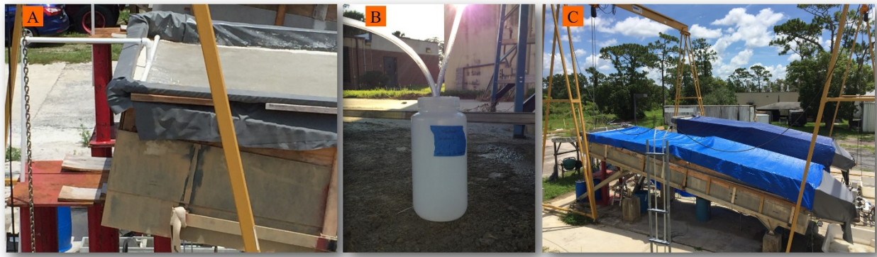
Figure 5. Roadway runoff delivered as sheet flow over pavement (A), collection of infiltrate samples (B), and models covered with waterproof tarpaulin to exclude natural rainfall (C).
