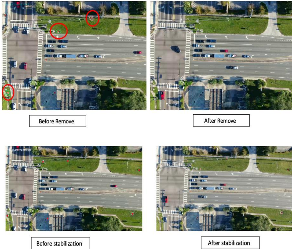
Figure 32 An example of result after removed objects that could cause a detection error
