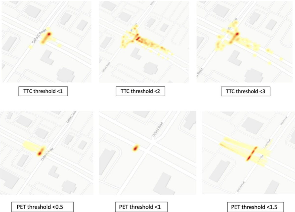
Figure 36 Vehicles' trajectories on PET and TTC values are less than 1.5 s in a 3D heatmap
