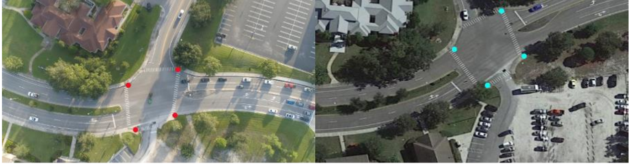
Figure 5 An example of converted pixel points for drone view and geographic map
