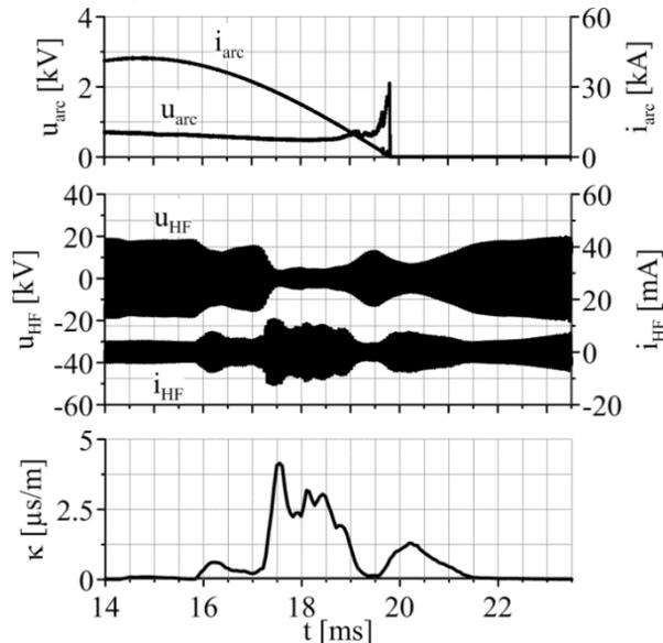
Fig.6: Example of measured signals and the calculated electrical conductivity
