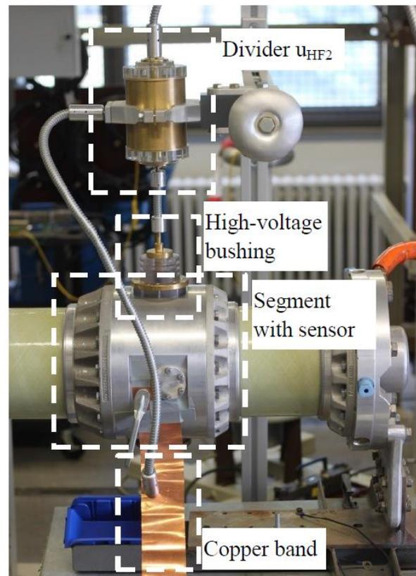
Fig.3: Specified SF<sub>6</sub> voltage divider and shielded Pearson Monitor (current transformer)
