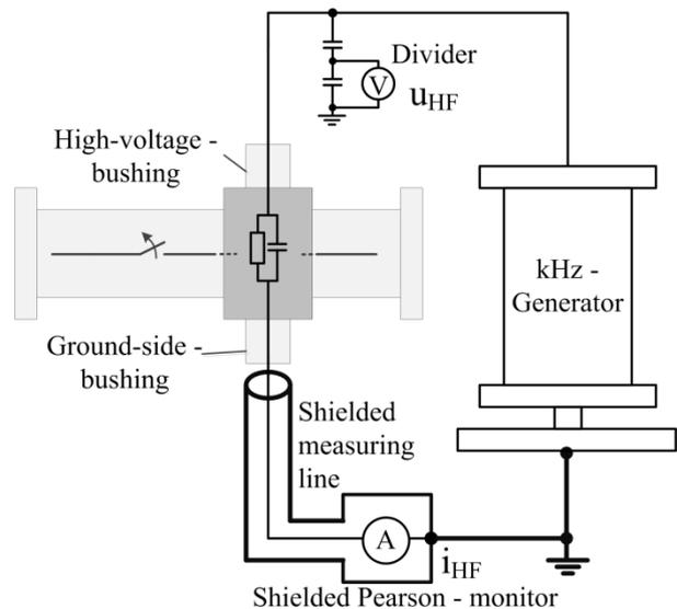
Fig.5: Measurement arrangement and the modified original SF<sub>6</sub>- circuit breaker
