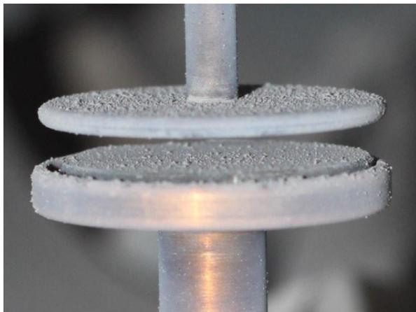
Fig.7: Polluted sensor after a few switching tests
