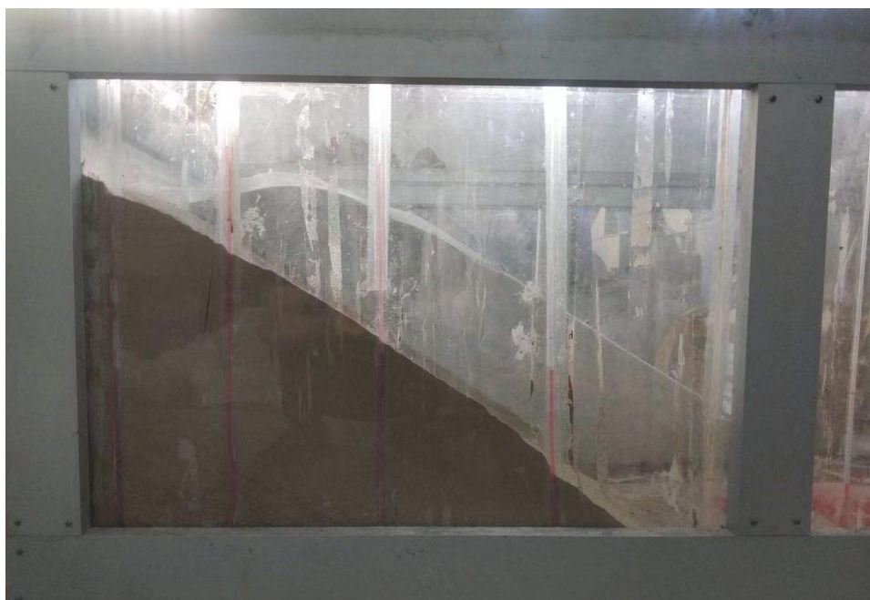
Fig. 4 – The experiment photo after the slope is formed (the condition: slope ratio = 1:1.5 and slope height =40cm)
