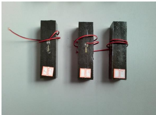
Fig. 3 - Polyurethane cement specimen
