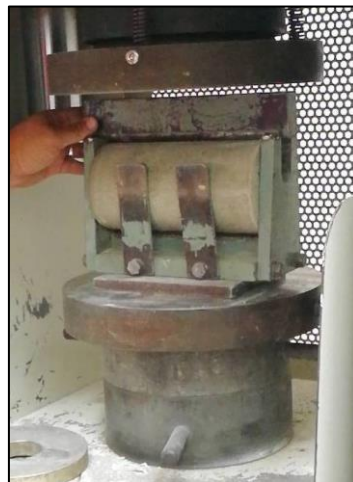
Fig. 7 - Splitting tensile test setup according to ASTM C496/C 496M
