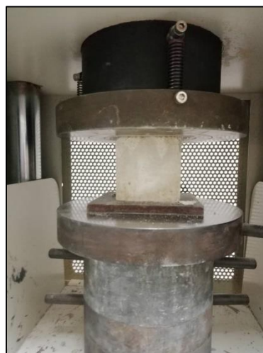
Fig. 5 - Compression test setup according to BS EN 12390-3: 2001
