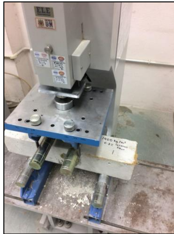
Fig. 6 - Flexural test setup according to ASTM C 348
