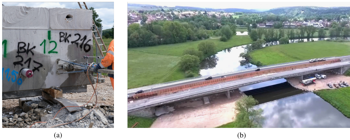
FIGURE 1. (a) Sampling of the drilling cores and (b) bird's eye view of the investigated bridge in Roding.
