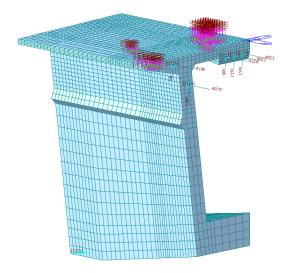
FIGURE 7. D model of cast-in situ pier elements.
