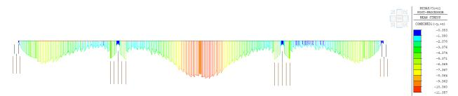
FIGURE 10. Sample of stress distribution in the top of deck (MPa) at time T=100y - quasi-permanent combination.
