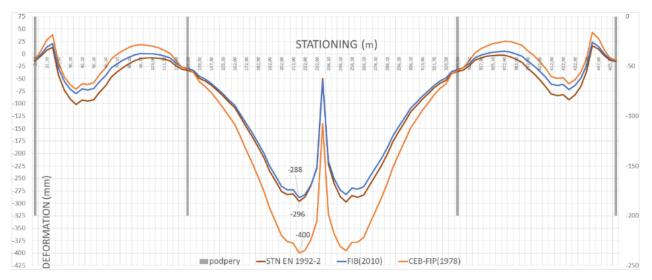
FIGURE 11. Deflections for different creep and shrinkage functions.
