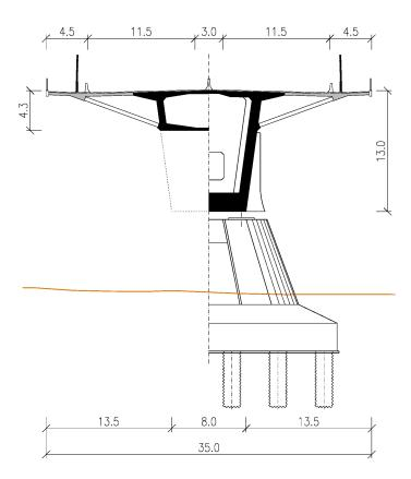
FIGURE 3. Cross-section in midspan and at piers.
