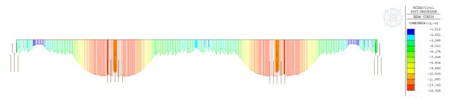
FIGURE 9. Sample of stress distribution in the bottom of deck (MPa) at time T=100y - frequent combination.
