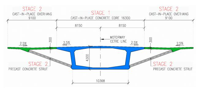
FIGURE 4. Deck cross-section construction stages.
