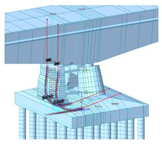
FIGURE 8. Model of temporary support at pier.
