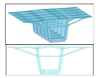
FIGURE 6. Shell element model.
