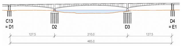
FIGURE 2. B Longitudinal section.
