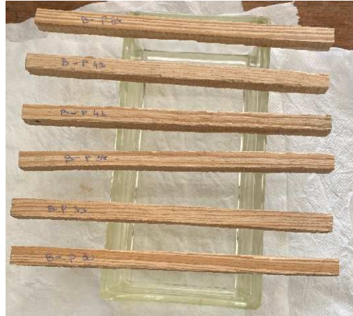
Figure 2: MW drying of the wood samples.
