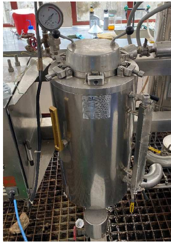
Figure 3: Autoclave used for the water impregnation.
