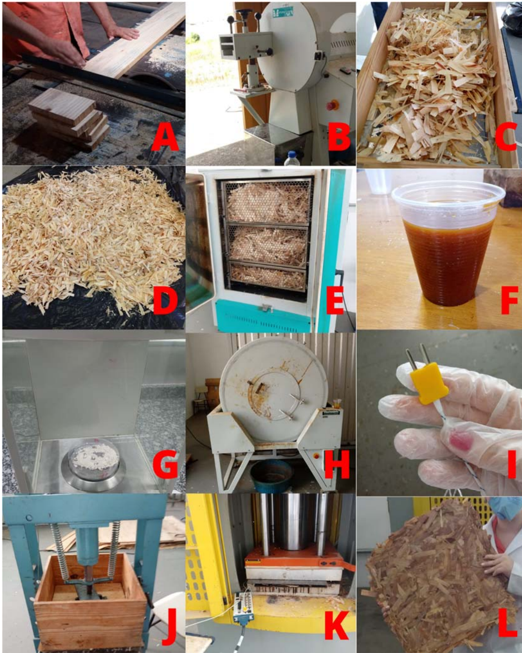
107 Figure 1: Production process of the boards. A: Wood processing; B: Wood chipping; C: Strands classification with 5 mesh shive; D: Natural drying of the strands; E: Oven 108 drying; F: Preparation of the adhesive; G: Weighing of nanoparticles H: Mixer-rotating 109 drum; I: Thermocouple type K; J: Pre-pressing; K: Hot pressing; L: Finished panel. 110
