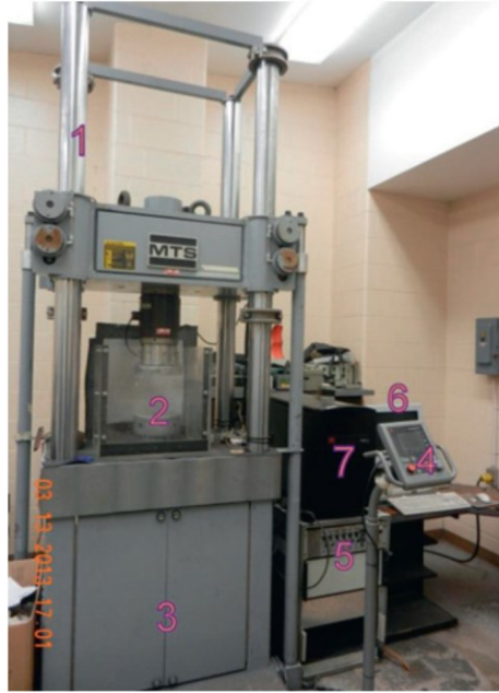
Fig. 3-9 MTS servo-controlled compression testing machine and its components (1) Machine load, (2) Glass shield, (3) Hydraulic actuator, (4) Manual control system, (5) Strain Gauge control panel, (6) Computer, (7) MTS data acquisition system (Xue, 2019)
