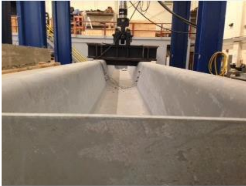
Figure 2.13: Initial Twist of Specimen #2 (Kelly, 2014)
