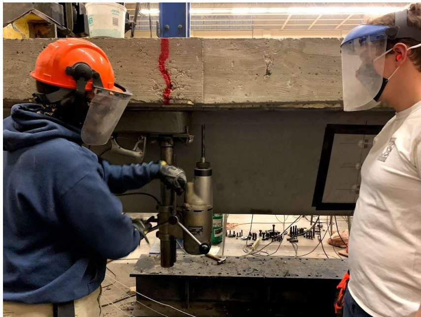
Figure 10.23: Drilling Through the PBFTG Top Flange
