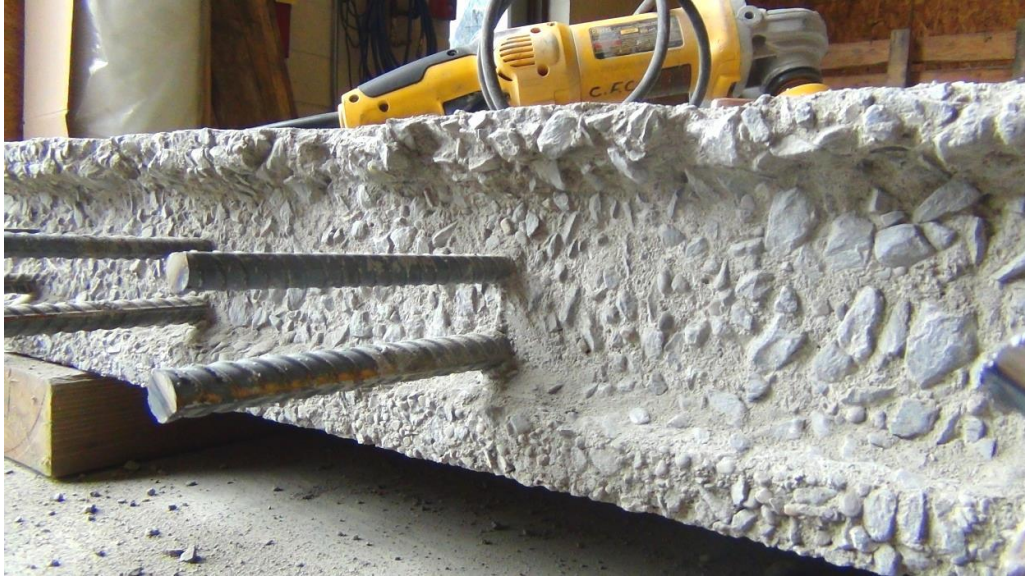
Figure 2.16: Concrete Surface after Wire-Brushing (Kozhokin, 2016)
