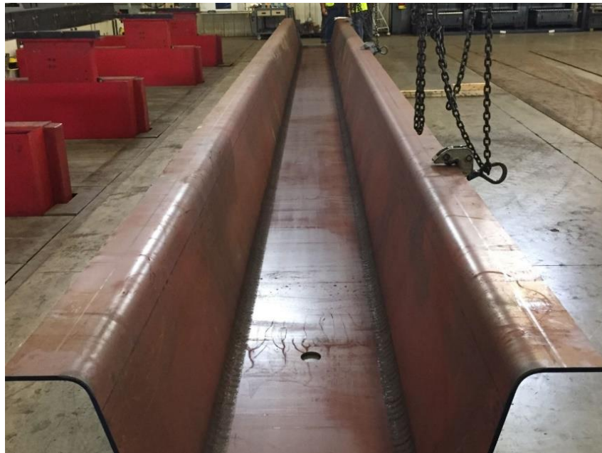
Figure 1.1: PBFTG after Cold Bending (SSSBA, 2021)
