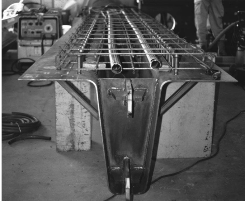
Figure 2.4: Negative Bending Test Specimen before Concrete Pour (Nakamura, 2002)
