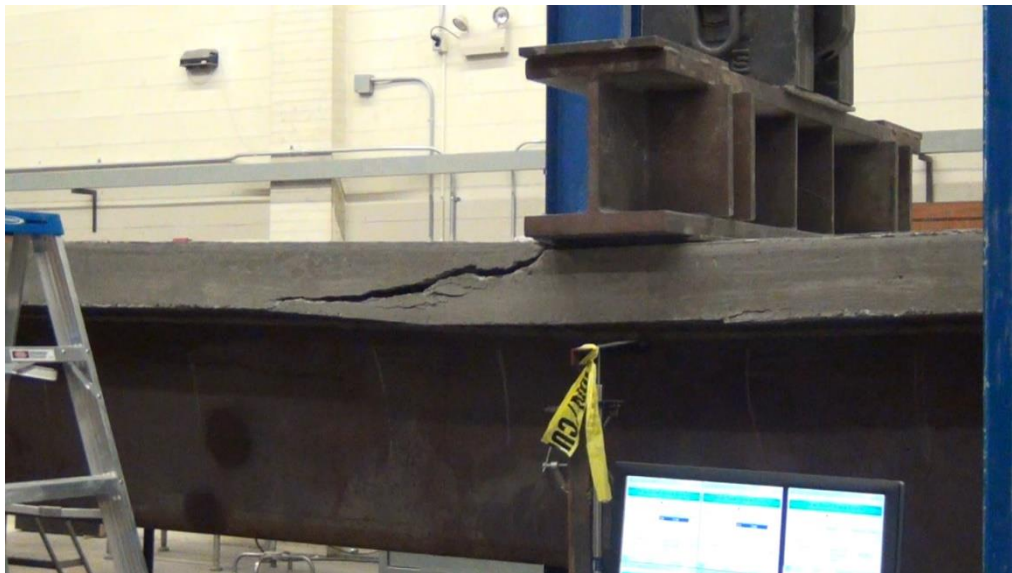
Figure 2.10: Typical Failure Mode for Composite Specimens (Michaelson, 2014)
