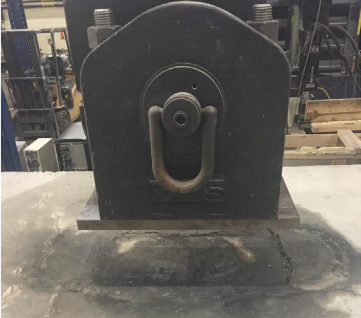
Figure 2.18: Concrete Deck Failure (Kozhokin, 2016)
