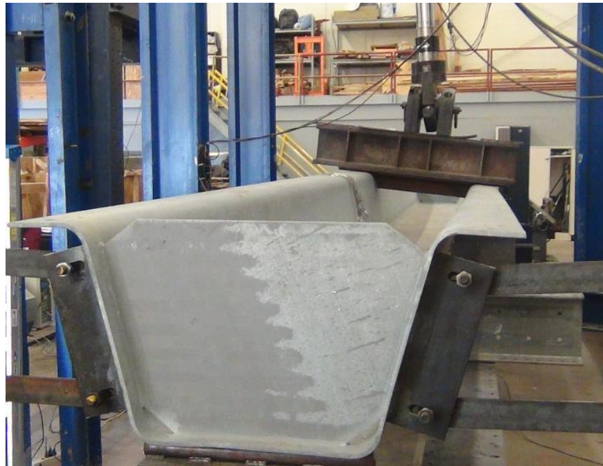
Figure 2.15: Lateral Torsional Buckling (Kelly, 2014)
