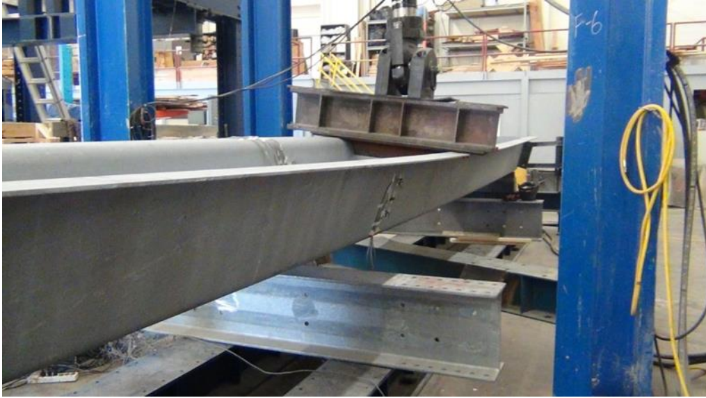
Figure 2.11: Typical Failure Mode for Noncomposite Specimens (Michaelson, 2014)
