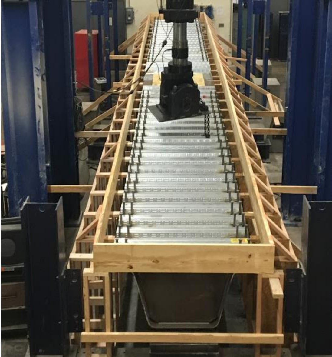
Figure 10.11: Isometric View of Complete Exterior Deck Forms
