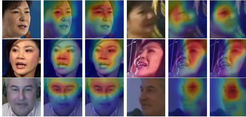
Figure 4.11: Class activation maps (CAMs) [3] with/without LANet module on three positive pairs from IJB-A quality dataset. Column 1 & 4: high- and low-quality faces of the same subject with various challenging factors (e.g. pose, illumination, blur, resolution and expression). Column 2 & 5: CAMs generated by SENet-HSNet model. Column 3 & 6: CAMs generated by Local and multi-Scale Convolutional Neural Networks (LS-CNN) model. Note that the fully connected layer before the final layer is removed in both models.
