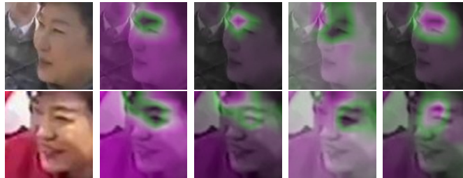
Figure 4.3: Four channels are visualized for a positive pair with similar eyes, where purple areas correspond to essential areas, and green areas mean less important ones. Different weights are assigned through the channel attention.
