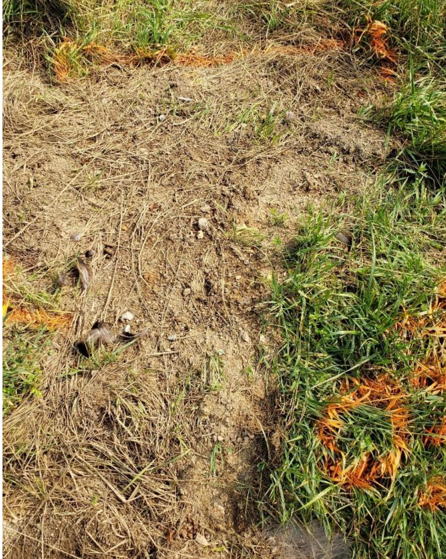
Figure 3. Example of training plot established to denote areas on pipeline that failed vegetative cover threshold. Plot is approximately 1m square and used a 2-digit identifier outside the bottom right corner
