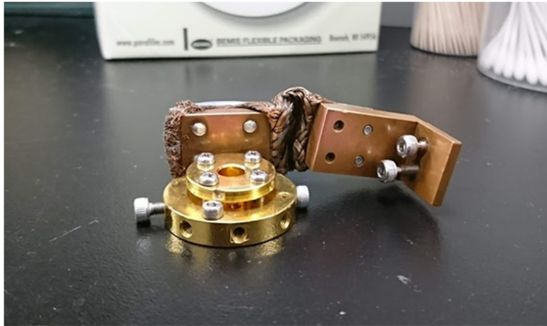
Figure 2-3 The sample holder for the cryogenic optical microscope system. The sample-holder surface was gold-coated with enhanced reflection to reduce the thermal conductance via the infrared radiation.
