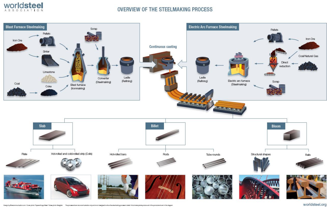
Figure. 1.2 Overview of the steelmaking process
