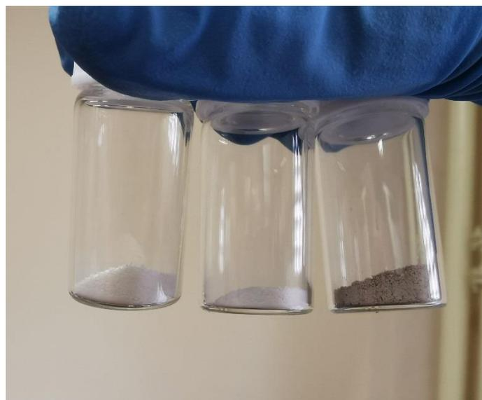
**Fig. 4.2.2.11.** The digital photograph of the as-synthesized pristine  $\text{TiO}_2$  (left),  $\text{TiO}_2\text{-air}$  (middle) and  $\text{OV s-TiO}_2\text{-N}_2$  (right), respectively.
