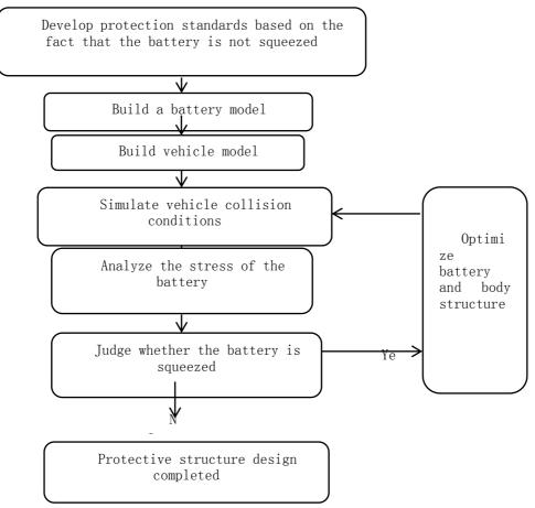
Figure 1 Traditional Protection Design Process
