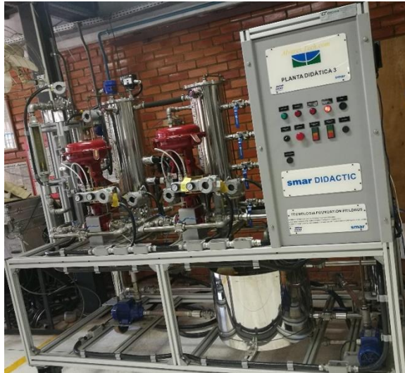
Figure 10. Smar Didactic Pilot Plant was used to develop the automatic tuning method. Source: authors.
