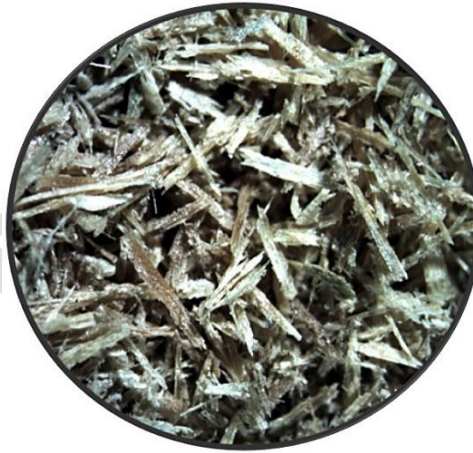
Figure 2. Stereoscopic Image (30X) of Musa acuminata US standard mesh No. 40 pseudostem particles. Source: authors.
