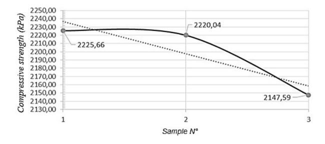
Fig. 5. Compressive strength in samples with 4% asphalt content. Source: Authors.
