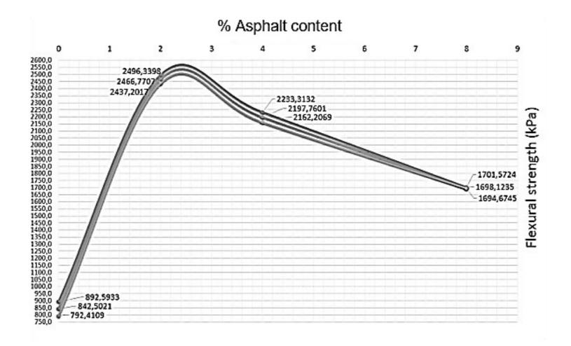
Fig. 15. Percentage of recycled asphalt vs flexural strength. Source: Authors
