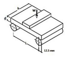
Fig. 8. Diagram of mounting module of rupture. Source: Authors.
