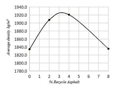
Fig. 2. Average densities according to recycled asphalt content. Source: Authors.
