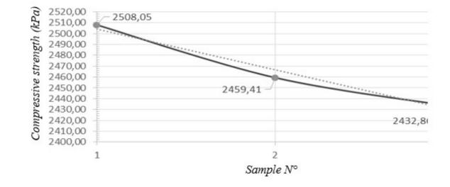
Fig. 4. Compressive strength in samples with 2% asphalt content. Source: Authors.
