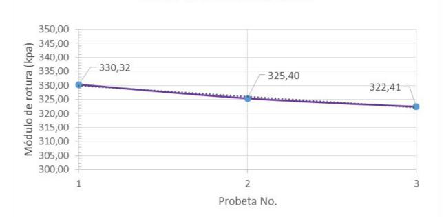
Fig. 11. Flexion strength in samples with 2% asphalt content. Source: Authors.
