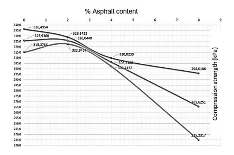
Fig. 14. Percentage of recycled asphalt vs compression strength Source: Authors.
