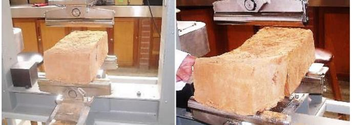
Fig. 9. Photographic record of flexural strength test. Source: Authors.
