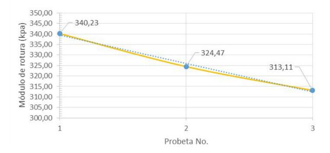
Fig. 10. Flexion strength in samples without asphalt content. Source: Authors.
