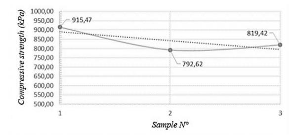
Fig. 3. Compressive strength in samples without asphalt content. Source: Authors.
