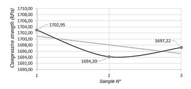
Fig. 6. Compressive strength in samples with 8% asphalt content. Source: Authors.
