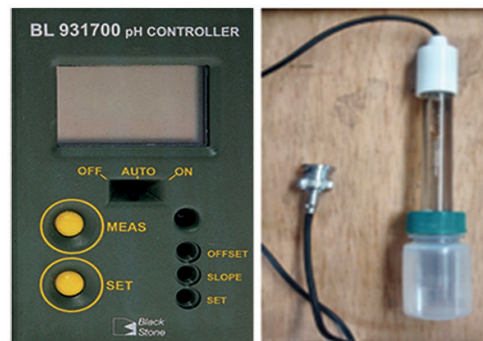
Fig. 5. Installed pH. indicator controller. Source: Authors
