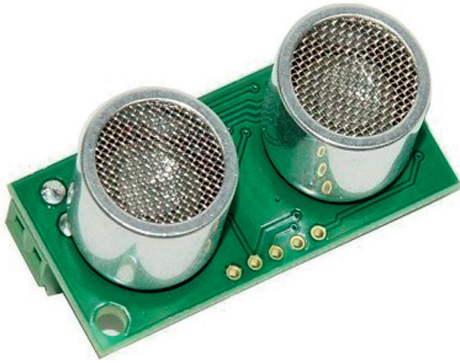
Fig. 8. Installed level sensor. Source: Authors
