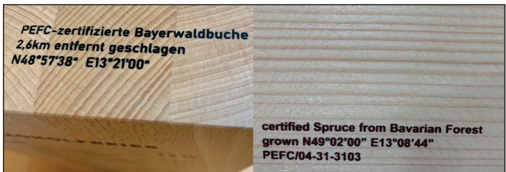
Figure 2: Coordinates of the felled timber: a bid to know the origin of the product.
