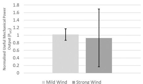
Figure 2: Comparison between the Useful Mechanical Power Output ( $P_{MO}$ ) normalised by means of the respective participant's Mild Wind (error bars refer to the standard deviation).
