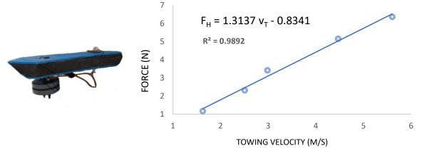
Figure 1: Hydrodynamic object (left) and experimental data used to create the model that predicts the resistance of the hydrodynamic object as a function of the towing velocity (right).
