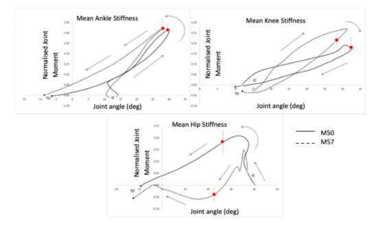
Figure 1. Joint moment-angle scatterplots for ankle, knee and hip – joint stiffness is represented as a gradient of the curve during stance. Grey dots – initial contact, black dots – toe off, red dots amortisation.
