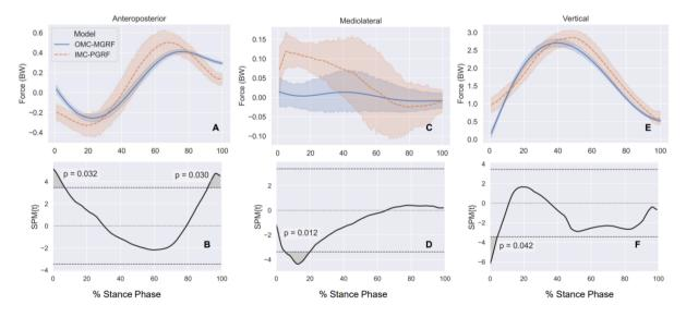
Figure 2: Mean and SPM plots presenting the GRF prediction for IMC-PGRF and the OMC-MGRF.
