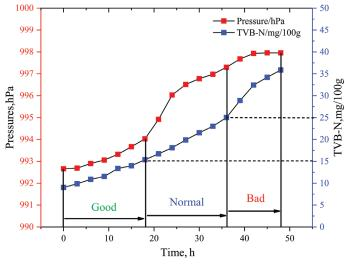
Figure 6. Correlation analysis of pressure and TVB-N of fish
