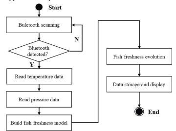
Figure 4. Workflow of the WPSS with freshness evolution of the fish
