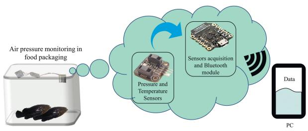
Figure 3. Experimental scheme of the WPSS for fish monitoring
