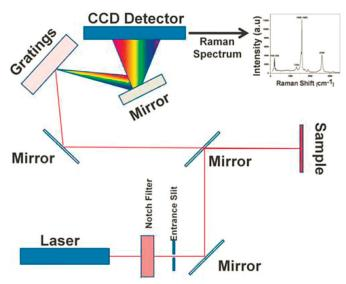
Figure 5. Principle scheme of the modern Raman spectroscope [36]
