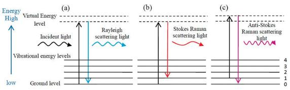
**Figure 4.** Diagram of the Rayleigh and Raman scattering processes: (a) Rayleigh scattering, (b) Stokes Raman scattering and (c) anti-Stokes Raman scattering [33]
