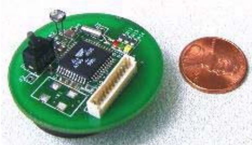
Figure 7 (b). Diagram showing actual size of a current generation Mote compared to one cent piece.
