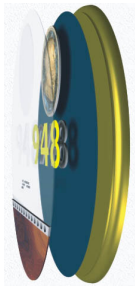
Figure 4.5 An 'exploded view' of BrailiantTouch® signage
