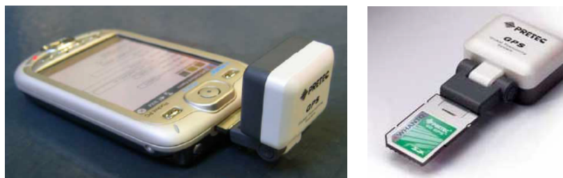
Figure 2a and 2b. The i-Mate PDA2k (a) with GPS receiver (b) attached in the SDIO card slot.
