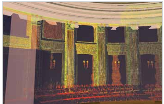
City Hall auditorium – laser scan superimposed over object-based model
