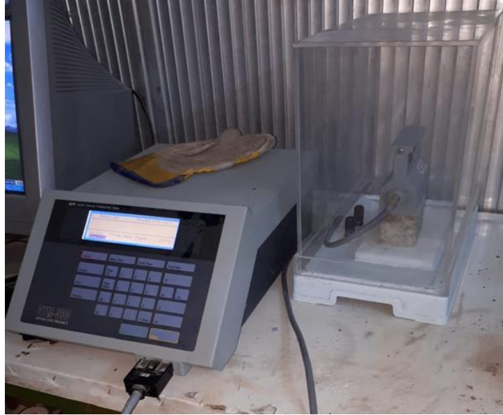
Figure 4. Thermal conductivity test device
