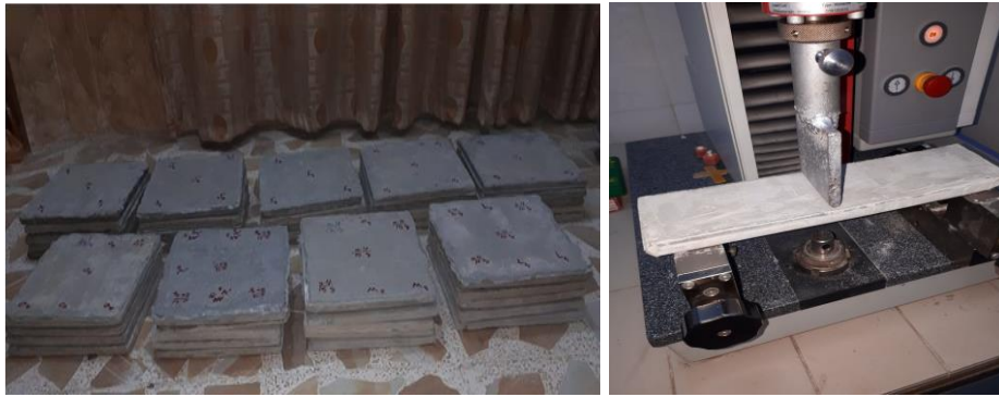
Figure 3. Sample and Flexural test device
