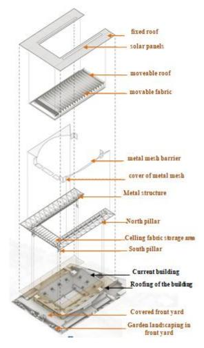
Figure 2. Shows the structural details on the roof of Lenglen tennis court [28]
