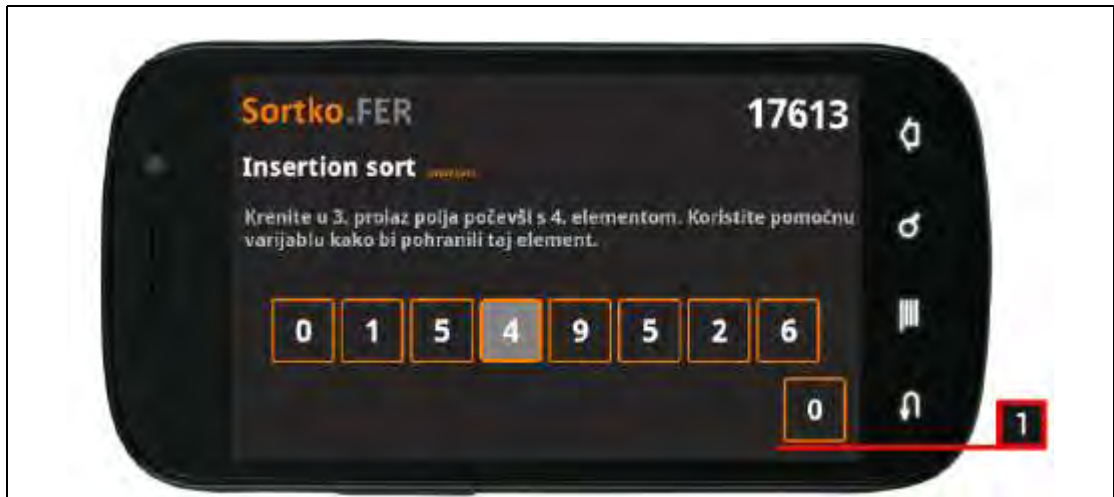
Figure 2.33. The Sortko mobile app, using switch elements to interact (Boticki, Barisic, Martin, and Drljevic, 2013)
