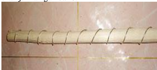
Gambar 6. Loading Sephasa Antena Vertikal 2 x 5/8 λ.
