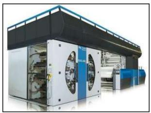
Fig. 3: Flexotecnica EVO XD Ten-Color Press (Source: Researcher)
