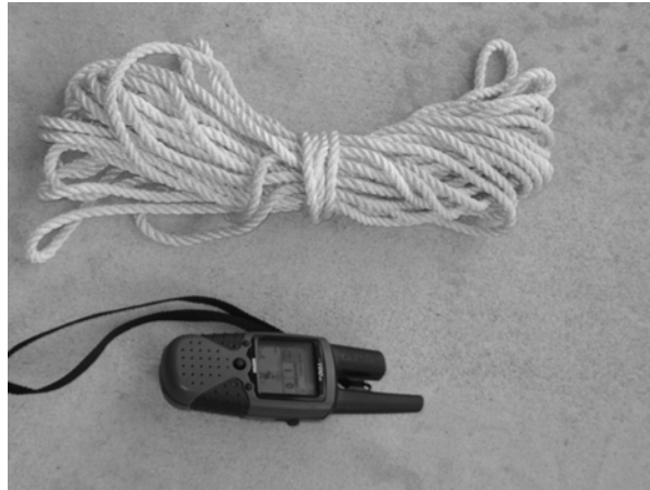
Figure 4: Two candidate pieces of equipment were used to determine the horizontal coordinate of points along the light path. The bottom device, a Global Positioning System receiver proved to be much less accurate than the rope shown on top.
