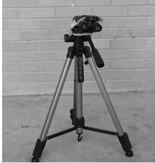
Figure 3: This device, consisting of a camera tripod with binoculars and laser points mounted on top, was used to aim and stabilize the light ray.
