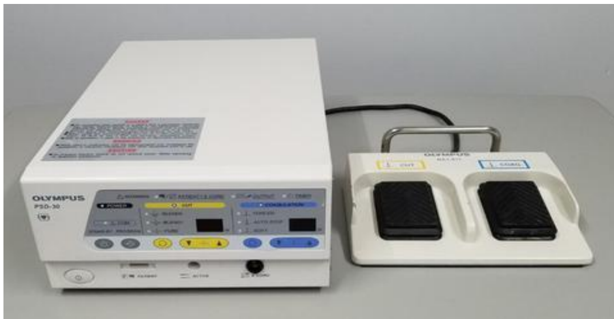
Figure 3. 1: Pictorial view of the Electrosurgical Unit (Primis Medical, 2021)
