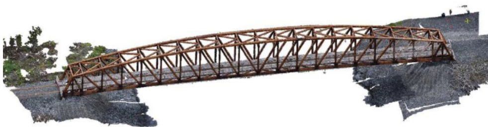
Figure 3.17 Alaska Center of Unmanned Aircraft System Integration point cloud reconstruction (dense structure-from-motion [SfM] techniques)
