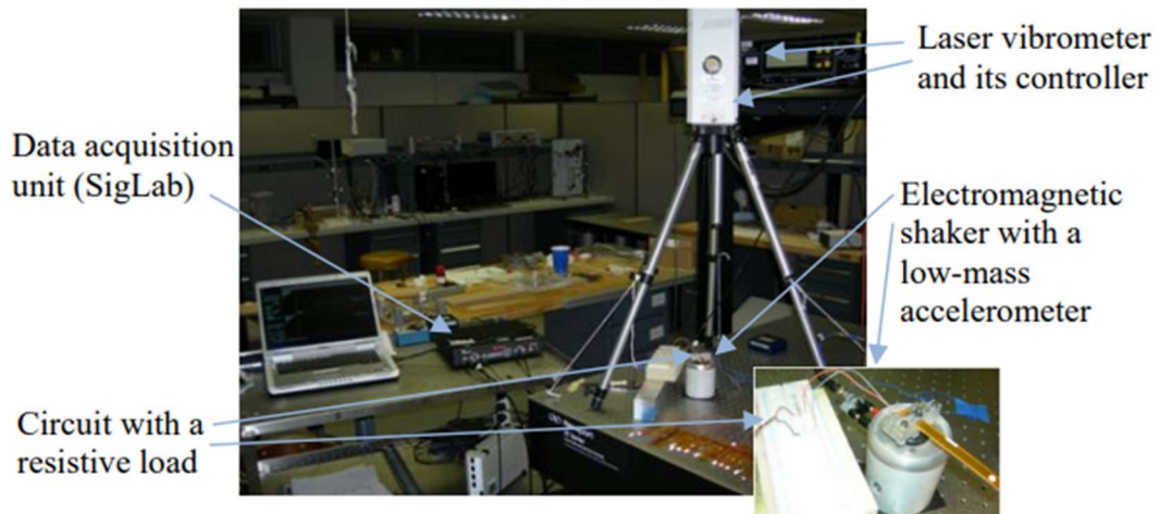
Fig 3.8. Experimental setup to test MFC Unimorph [13]
