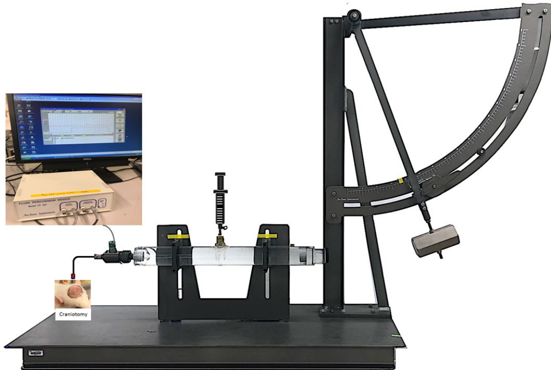
Figure 1.1 Fluid percussion injury model. The fluid pulse impacts at the exposed dura by craniotomy. Source: [25].
