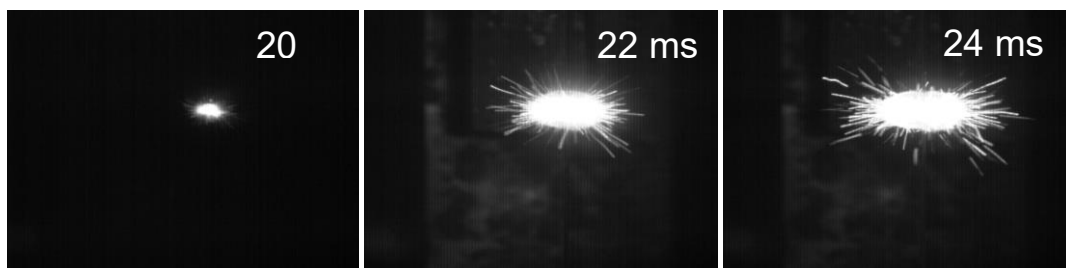
Figure 2.9 A characteristic sequence of video frames showing ignition of S4 (milled in 25% ACN). Heating rate is 34700 \pm 1500 K/s.
