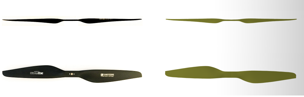
Fig. 1 Top and front views comparison between original blade(Left) and reconstructed CAD model(Right).
