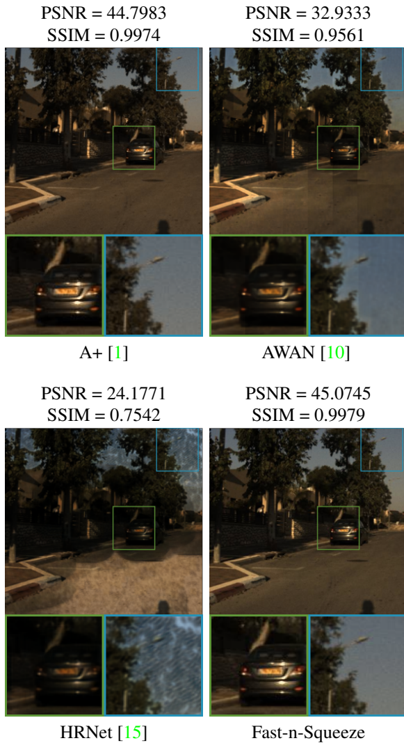
Figure 5. Comparison of some details of the reconstructed images with the considered methods. The images are obtained by applying Eq. 2 to the generated spectral images.
